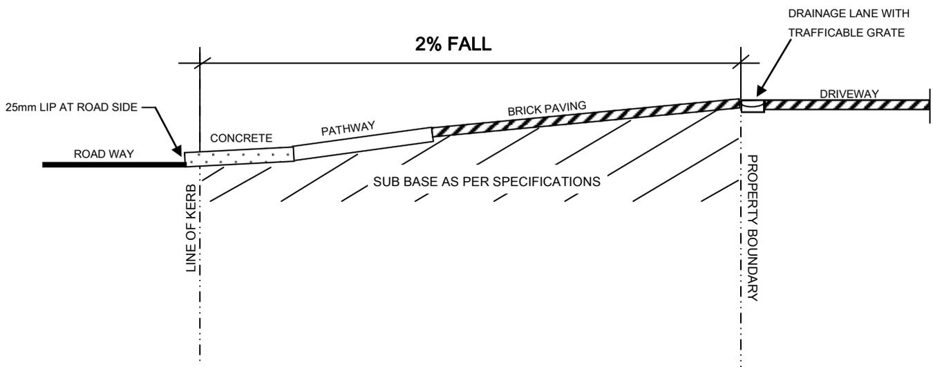
**2% Fall taken from the top of the paving at the property boundary to the top of the kerb at the road side.**
